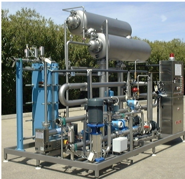
Combination Deaeration, Chilling, Blending & Carbonation System
