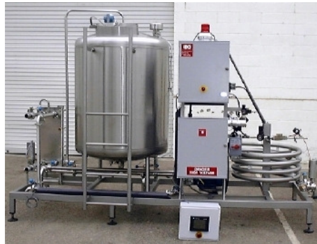
In-line Carbonation System
